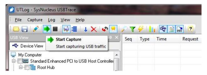
Insert your dongle in the USB port and in the USBTrace window you should see the log:
